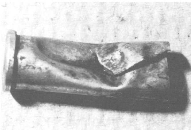
FIG. 3A—Basilar view of the "live" cartridge recovered from the right temporal lobe at autopsy; note absence of markings or indentations on the head stamp, and B—lateral, exterior view of the casing with distorted contour in area of rupture and patches of lead smears.
